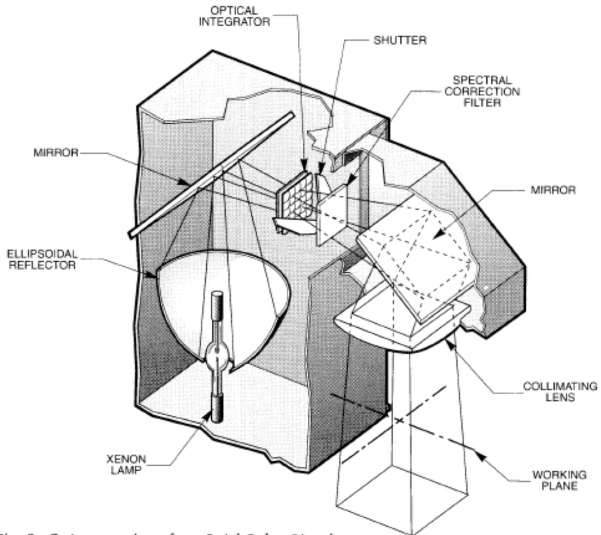
Fig. 2 Cut-away view of an Oriel Solar Simulator.
